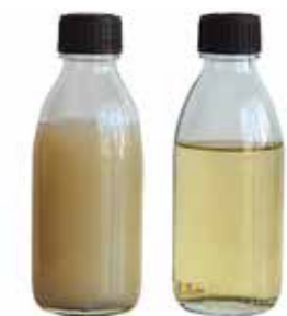
Process oil at a German manufacturer of common-rail injection systems before and after recycling
