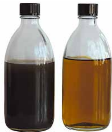
Process oil at a German premium automobile manufacturer before and after recycling
