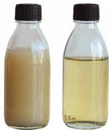
Process oil at a German manufacturer of common rail injection systems before and after recycling
